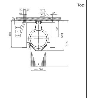
**Electric** Supply voltage: 230 V/1 ph/50/60 Hz Total Watts: 0.2 kW Steam Steam generation: External source Steam inlet size: Steam pressure Max: 1.5 bar Steam supply, relative dynamic pressure: 1 min bar, 1.5 max bar Water: Pressure, min-max: 2-6 bar Installation:
